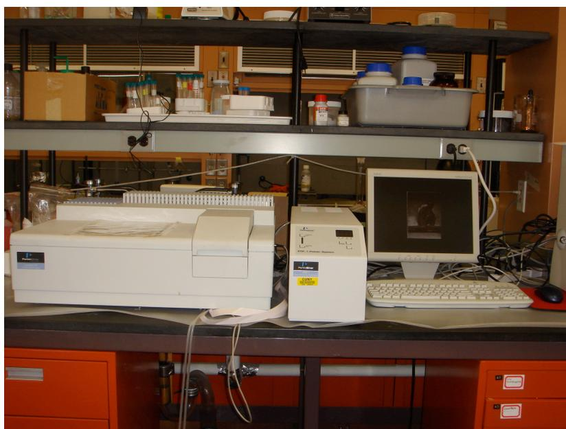
**Scheme 8 Perkin- Elmer Lambda 25 UV-Vis spectrophotometer used in the experiment**
