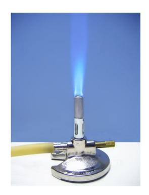
**INSPECT** hose for cracks, holes, pinched points, or any other defect, and ensure that the hose fits securely on the gas valve and the Bunsen burner. **Replace** all hoses found to have a defect before using.
