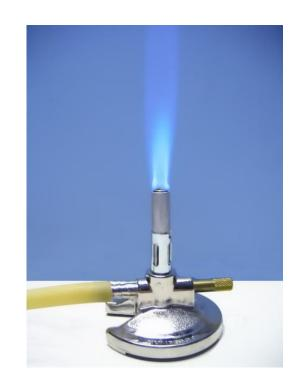
**DO NOT** leave open flames unattended and never leave laboratory while burner is on and do not use Bunsen burners in biological safety cabinets.
