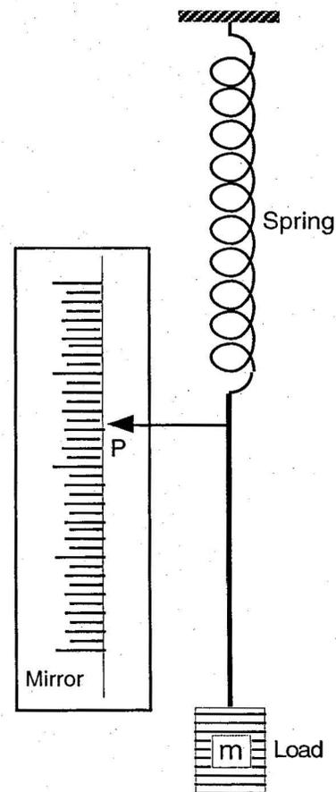
If the load on the spring is  $M$  and  $M_p$  is the sum of the mass of the hanger and the effective mass of the spring,  $F_{\text{ext}} = (M+M_p)g$ . In this experiment, values of  $x$  for a number of values of  $F_{\text{ext}}$  are determined by changing  $M$ . Then a graph of  $M$  vs.  $x$  is plotted and  $k$  is determined from the slope of the graph.
