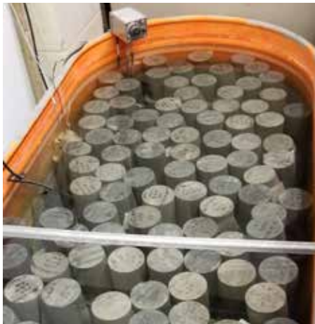
Representative drilled core samples prepared to undergo geotechnical tests to assess the subsoil load-bearing capacity.
