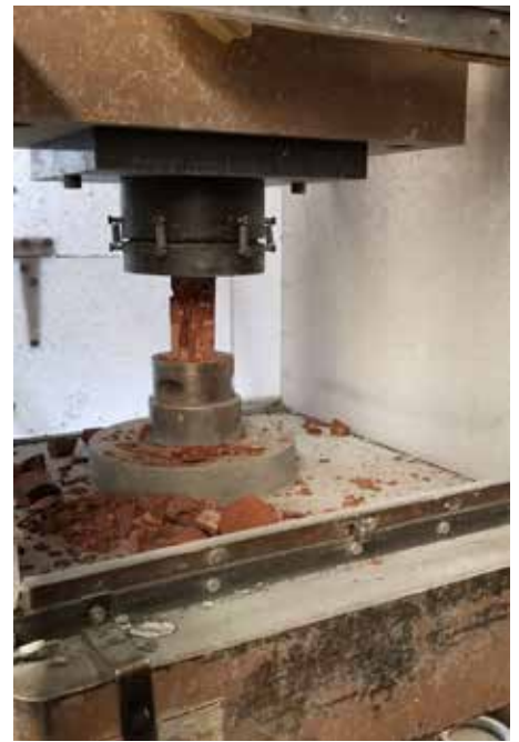
Concrete strength measuring tool. Also ideal for rock core compression tests routinely needed for determining foundation strength concerning load-bearing capacity.
