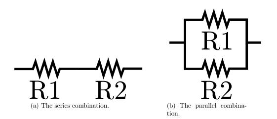
Figure 6: Series and parallel resistance combinations.
