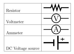
Table 1: The various schematic elements used in this lab.
