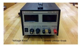
Figure 2: The direct current power supply.
