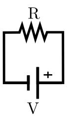
Figure 1: The simplest direct current circuit.
