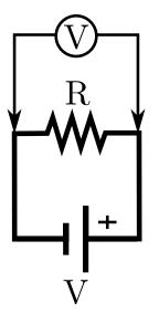
Figure 4: The simplest direct current circuit, with voltmeter installed.
