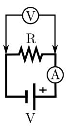
Figure 5: The direct current circuit with ammeter inserted.
