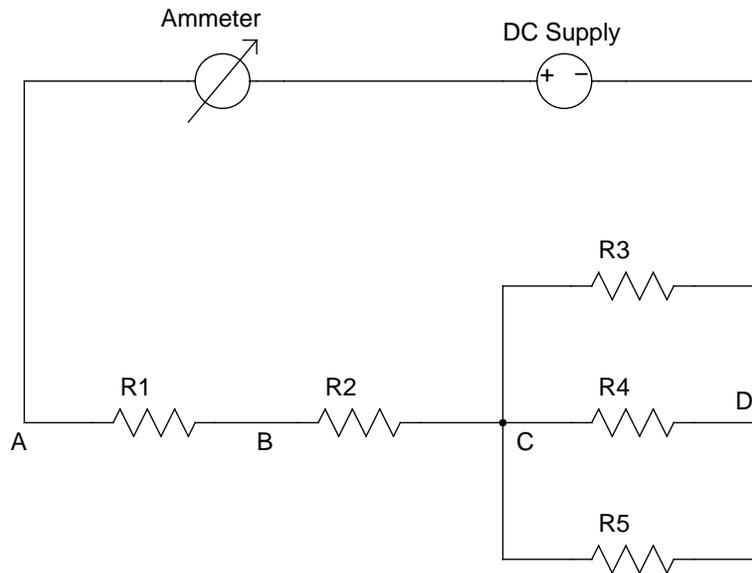
Figure 3: The circuit used to test the parallel and series resistance combinations.
