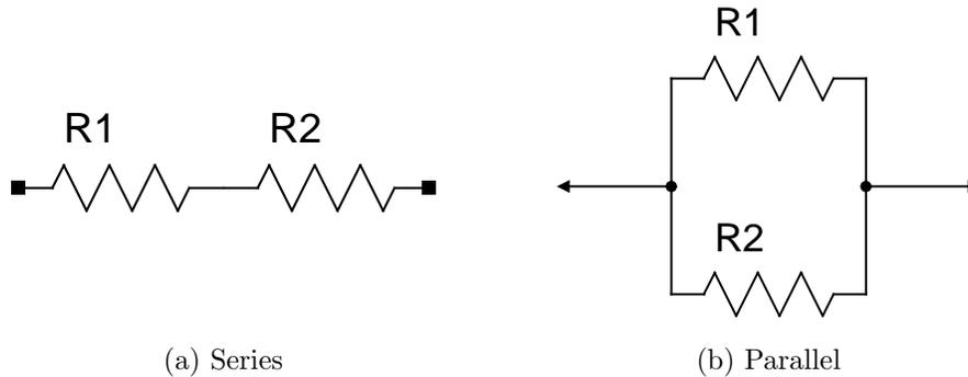
Figure 2: Series and parallel resistor configurations.
